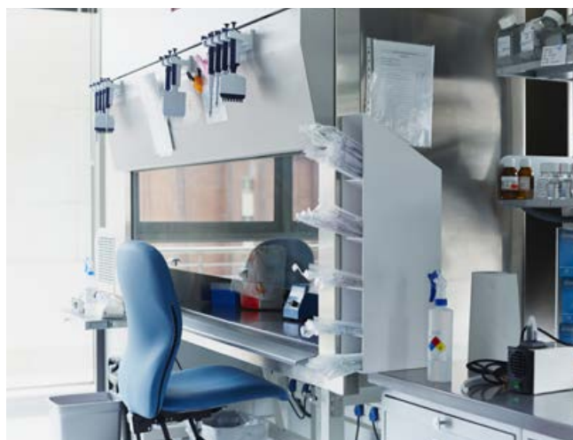
Laboratory fume hood
