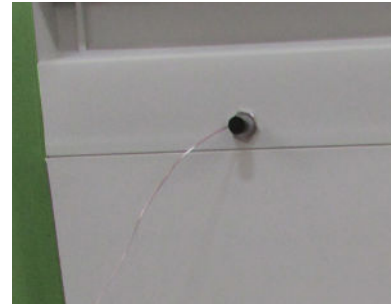
Thermocouple through Access Port &amp; Access Port Plug.
