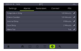
Once the Alarm Test window opens, press 'Start Test' to activate the fault signal on the external relays. Confirm the attached monitoring system sees a fault.
