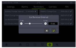
Select 'Ice Removal Due' to acknowledge the ice has been removed from the freezer in the gasket area and update the due date.
