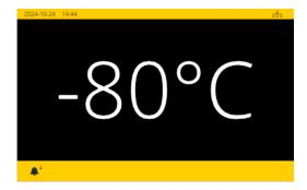
Tapping the alarm/alert bell leads to an Active Notifications screen. Alarms are displayed with a red indicator; alerts have a yellow indicator.
