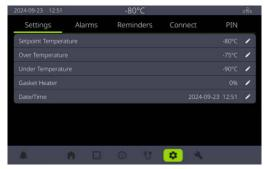
Gasket Heater screen allows users to change the gasket heater duty cycle from 0% to 100%. Increase the percentage for more defrost heating when there is ice buildup around the door.
