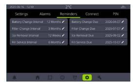
Adjust interval to an appropriate setting for your circumstances. Ice stops the freezer from optimum performance. Ice build-up decreases uniformity and increases power consumption.
