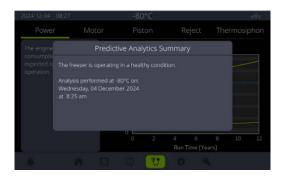
Power: Charts Engine Power (Watts) vs. Run Time (Years) to determine if the engine power consumption is within the expected range.
