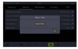
Press the 'Stop Test' button to disengage the fault signal. Confirm the attached monitoring system clears the fault note. (NOTE: An actual fault will override this signal, continuing to show fault on the dry contact output.)
